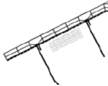
J HOOK ENGAGED TO TENDON FOR TENSION
